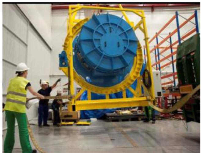
Fig. 12. EMIR cryostat on the AIV and transport structure.
